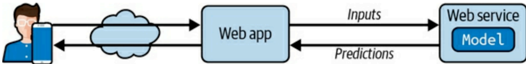
Figure 2-20. A model deployed as a web service and used by a web application
