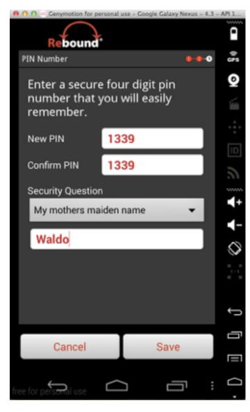
platform-tools \$./adb logcat | grep encod D/update ( 3350): encodedXmlData-->%3c%3fxm %3e%3cPin%3e1339%3c%2fPin%3e%3c%2fSettings%3 D/YGIB Test( 3350): content-->%3c%3fxml%20ve Pin%3e1339%3c%2fPin%3e%3c%2fSettings%3e%3c%2
