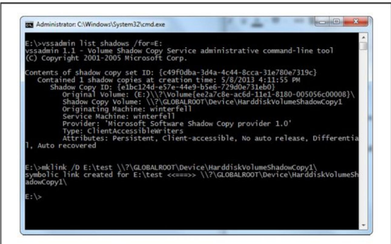
Figure 12-7. Syntax to list shadow copies for a volume and mount via symbolic link
